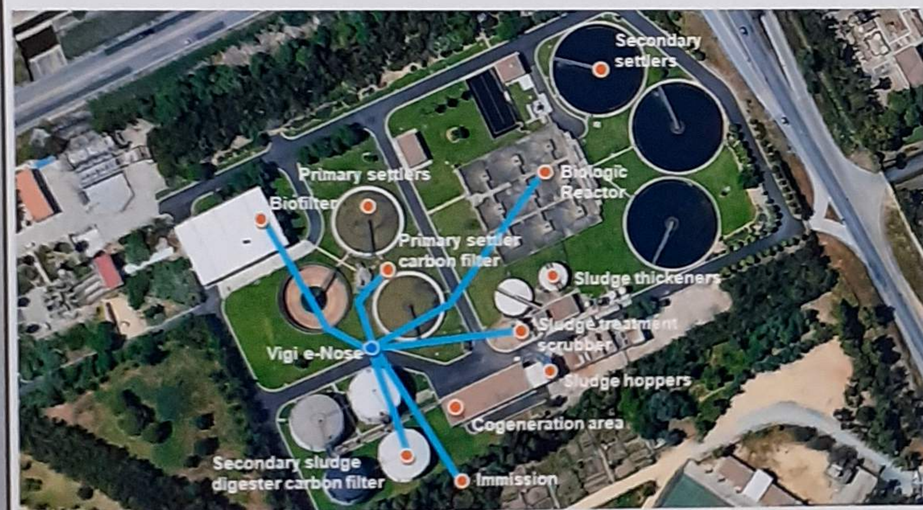
Figure 1: Emission sources and connections to the Vigi e-Nose analyser
